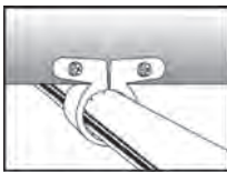
Install with screws to metal studs.
