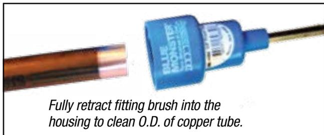
*Fully retract fitting brush into the housing to clean O.D. of copper tube.*
