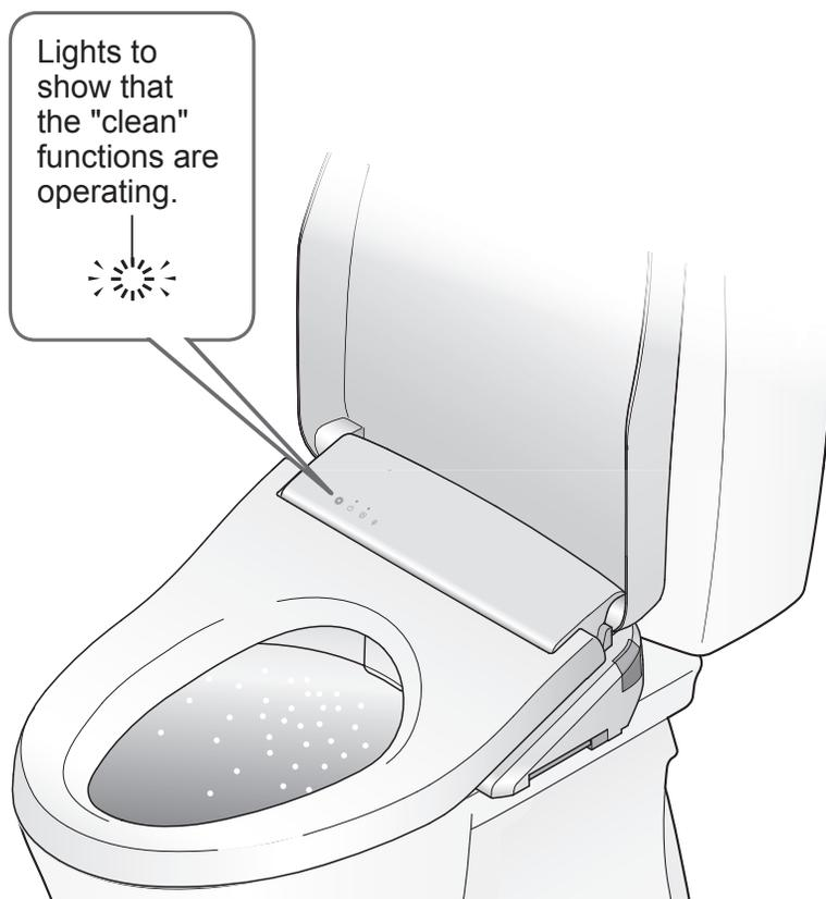
The self-cleaning functions operate automatically.
